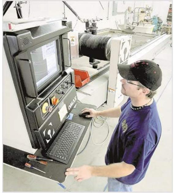
Operator Rodney McDonald makes programming adjustments on the OMAX 80160 Waterjet Machining Center, a new cutting device at Neosource.
